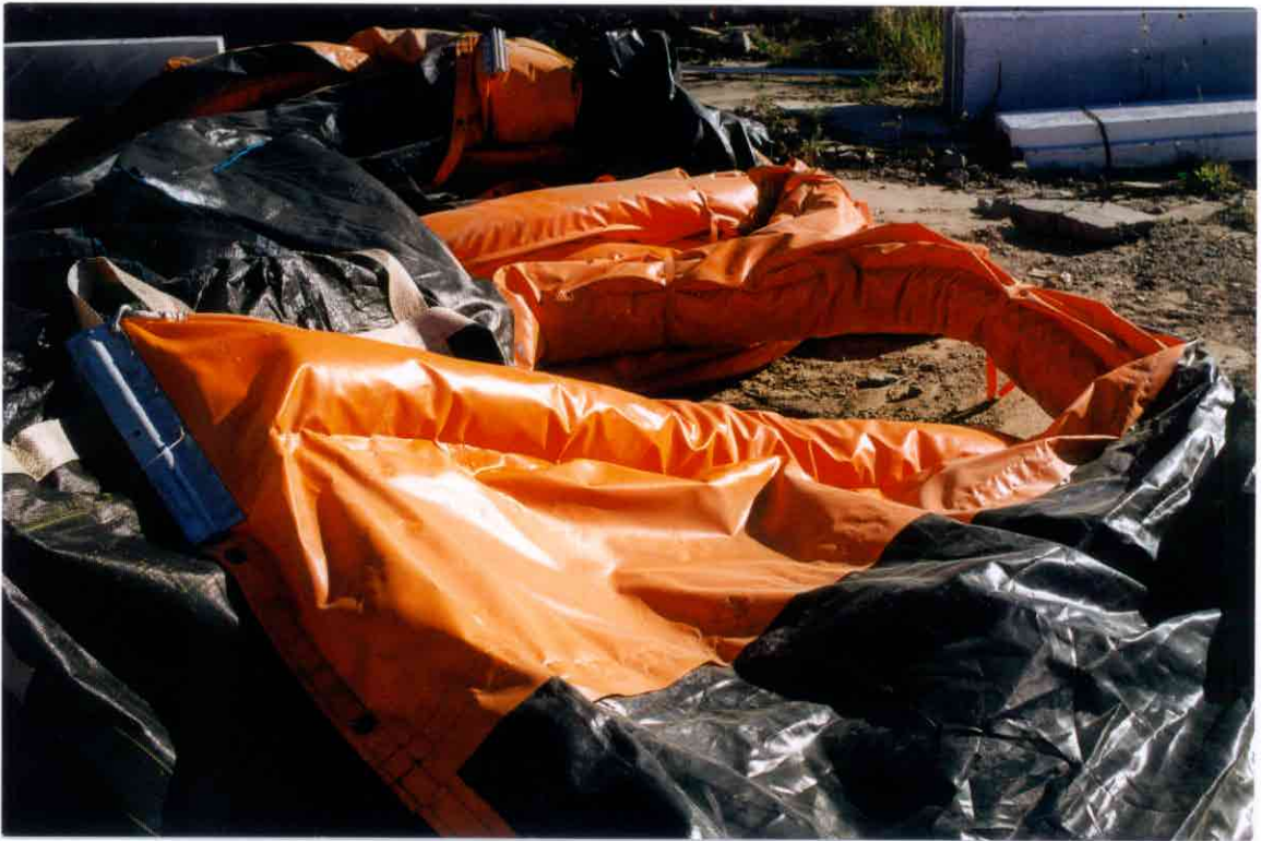
Photo No. 1: Spare silt curtain panel. Note orange floatation, black silt curtain skirt, and slide connector.
