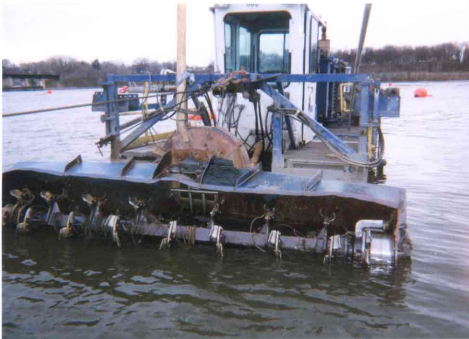
Photo No. 4: Horizontal auger cutterhead on IMS 4010 Versi-Dredge.
