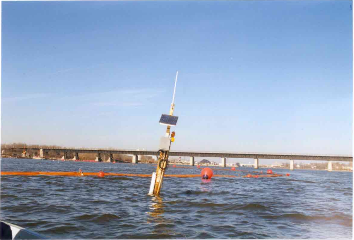
Photo No. 19: Real-time turbidity monitor on piling at the SSO position. Note the radio antenna, solar panel, data collection box, electric cabling, flasher light, and PVC pipe containing the turbidity sensor.
