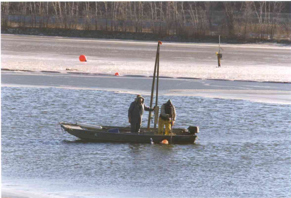
Photo No. 22: Measuring water depth before collecting a post-dredge sediment core sample. Note sample tube in boat and pipe in water marking the pre-dredge core location.
