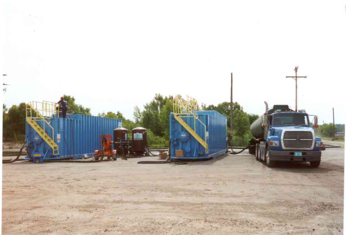
Photo No. 26 Portable water treatment system used during clean out of the equalization basins and demobilization activities.
