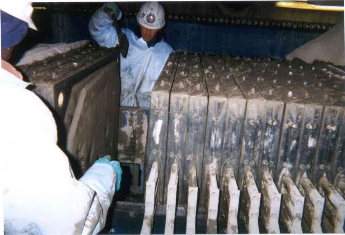
Photo No. 13: Filter cake being removed from press plates
