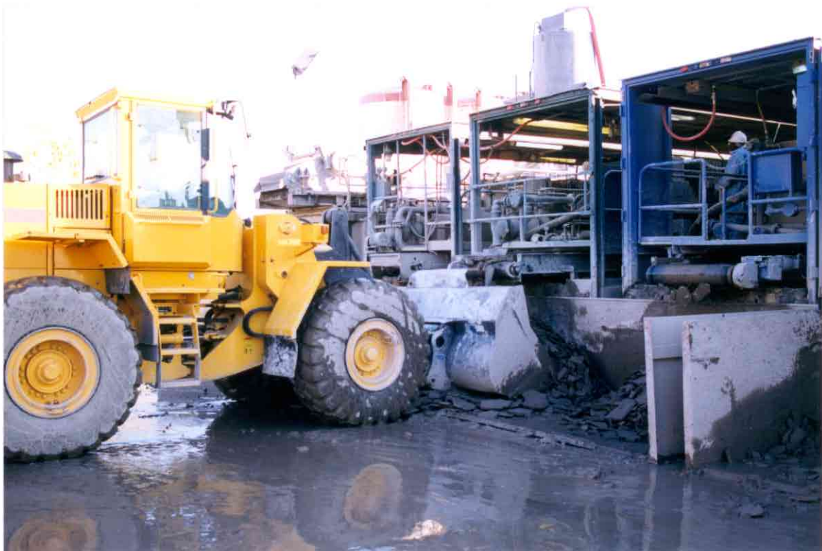
Photo No. 14: Front-end loader removing dewatered sediment from press bins.
