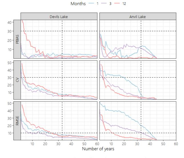
**Figure A10. Time series length sensitivity of the coefficient of variation in the rate of lake level rise.** Bias (PBIAS), precision (CV), and accuracy (RMSE) for each lake for the coefficient of variation in rate of lake level rise over 1 month, 3 months, and 12 months. Dashed vertical lines correspond to a 33-year time series. Dashed horizontal lines represent a PBIAS of 30%, CV of 30%, and RMSE of 10%.
