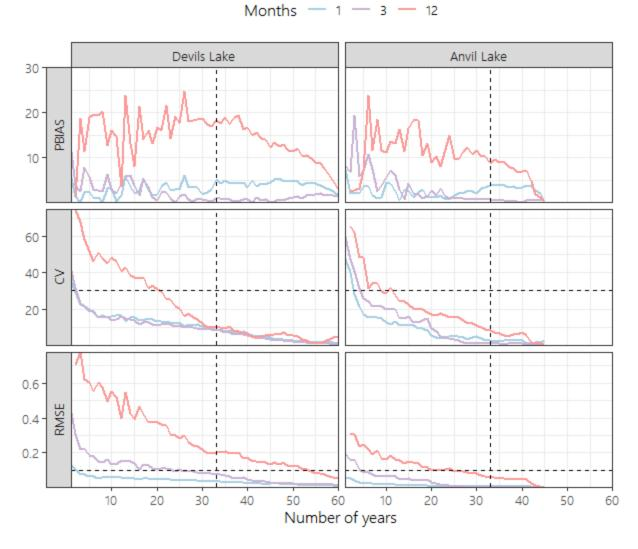
**Figure A11. Time series length sensitivity of the median rate of lake level fall.** Bias (PBIAS), precision (CV), and accuracy (RMSE) for each lake for the median rate of lake level fall over 1 month, 3 months, and 12 months. Dashed vertical lines correspond to a 33-year time series. Dashed horizontal lines represent a PBIAS of 30%, CV of 30%, and RMSE of 0.1 ft
