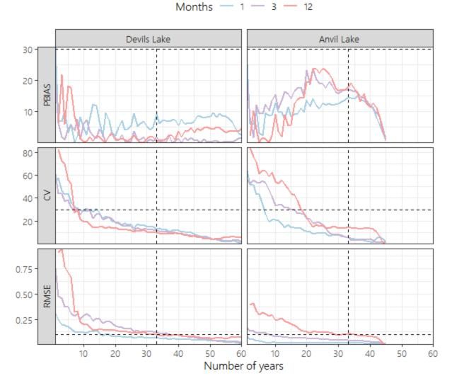
**Figure A9. Time series length sensitivity of the median rate of lake level rise.** Bias (PBIAS), precision (CV), and accuracy (RMSE) for each lake for the median rate of lake level rise over 1 month, 3 months, and 12 months. Dashed vertical lines correspond to a 33-year time series. Dashed horizontal lines represent a PBIAS of 30%, CV of 30%, and RMSE of 0.1 ft.
