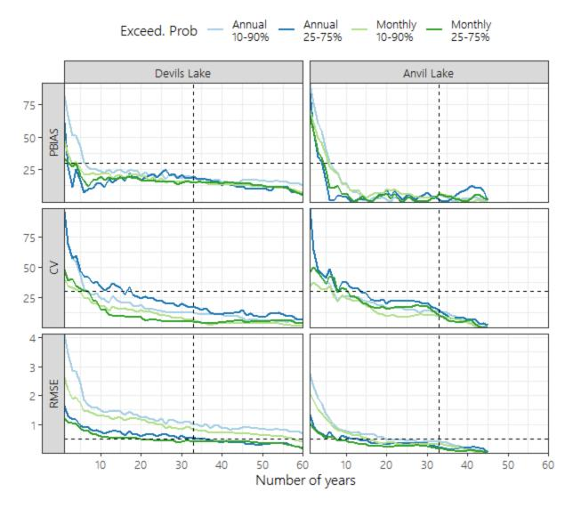
**Figure A4. Time series length sensitivity of ranges in lake levels.** Bias (PBIAS), precision (CV), and accuracy (RMSE) for each lake for the range in lake levels between the 10% and 90% exceedance probabilities and 25% and 75% exceedance probabilities calculated with all monthly lake levels ("monthly") and with annual mean lake levels ("annual"). Dashed vertical lines correspond to a 33-year time series. Dashed horizontal lines represent a PBIAS of 30%, CV of 30%, and RMSE of 0.5 ft.
