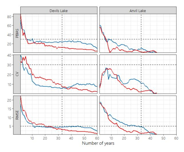
**Figure A6. Time series length sensitivity of percent of time lake levels are within 1ft of median levels.** Bias (PBIAS), precision (CV), and accuracy (RMSE) for each lake for the percent of time lake levels are within +1ft or -1ft of the median. Dashed vertical lines correspond to a 33-year time series. Dashed horizontal lines represent a PBIAS of 30%, CV of 30%, and RMSE of 5%.
