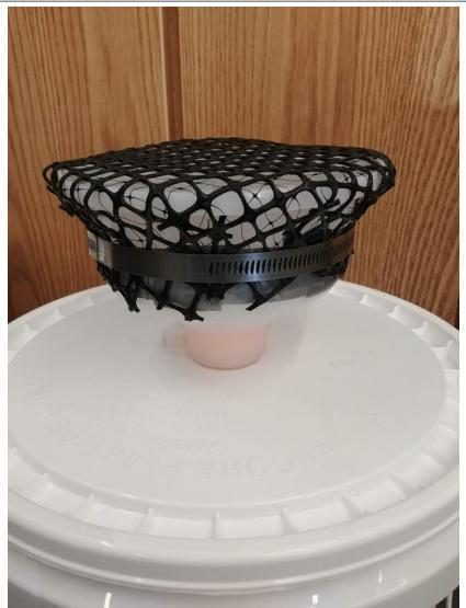
**Figure 12. Precipitation collectors.** Water passes through the plastic mesh and past the buoyant ping-pong ball to the 4-liter jug nested inside the bucket.
