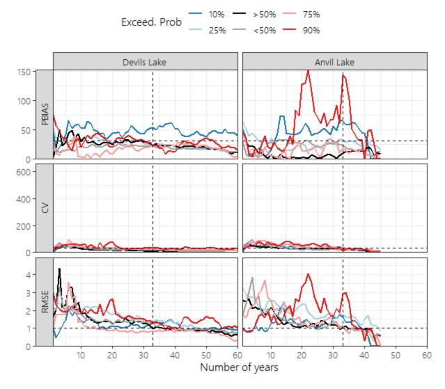
**Figure A7. Time series length sensitivity of median duration of high/low lake levels.** Bias (PBIAS), precision (CV), and accuracy (RMSE) for each lake for the median duration at/above the 10%, 25%, 50% and 50% + 1 ft. exceedance probability levels or at/below the 50%, 50% - 1 ft., 75% and 90% exceedance probability levels. Dashed vertical lines correspond to a 33-year time series. Dashed horizontal lines represent a PBIAS of 30%, CV of 30%, and RMSE of 1 month.
