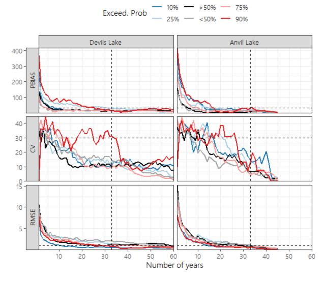
**Figure A5. Time series length sensitivity of frequency of high/low lake levels.** Bias (PBIAS), precision (CV), and accuracy (RMSE) for each lake for the number of times lake levels are at/above the 10% and 25% exceedance probability levels or at/below the 75% and 90% exceedance probability levels per decade. Dashed vertical lines correspond to a 33-year time series. Dashed horizontal lines represent a PBIAS of 30%, CV of 30%, and RMSE of 1 time/decade.
