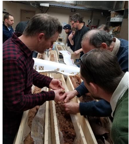
WGNHS and DNR staff examine rotosonic core from central Wisconsin, collected as part of the central sands lakes study. Photo: Ken Bradbury
