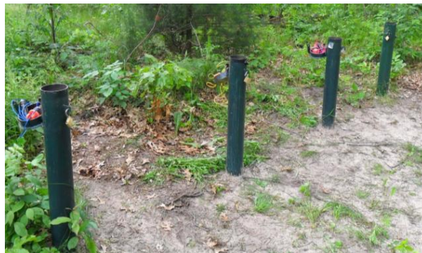
Nested piezometers installed for monitoring groundwater levels and sampling for groundwater contaminants near Spring Green. Photo: Blake Russo-Nixon.
