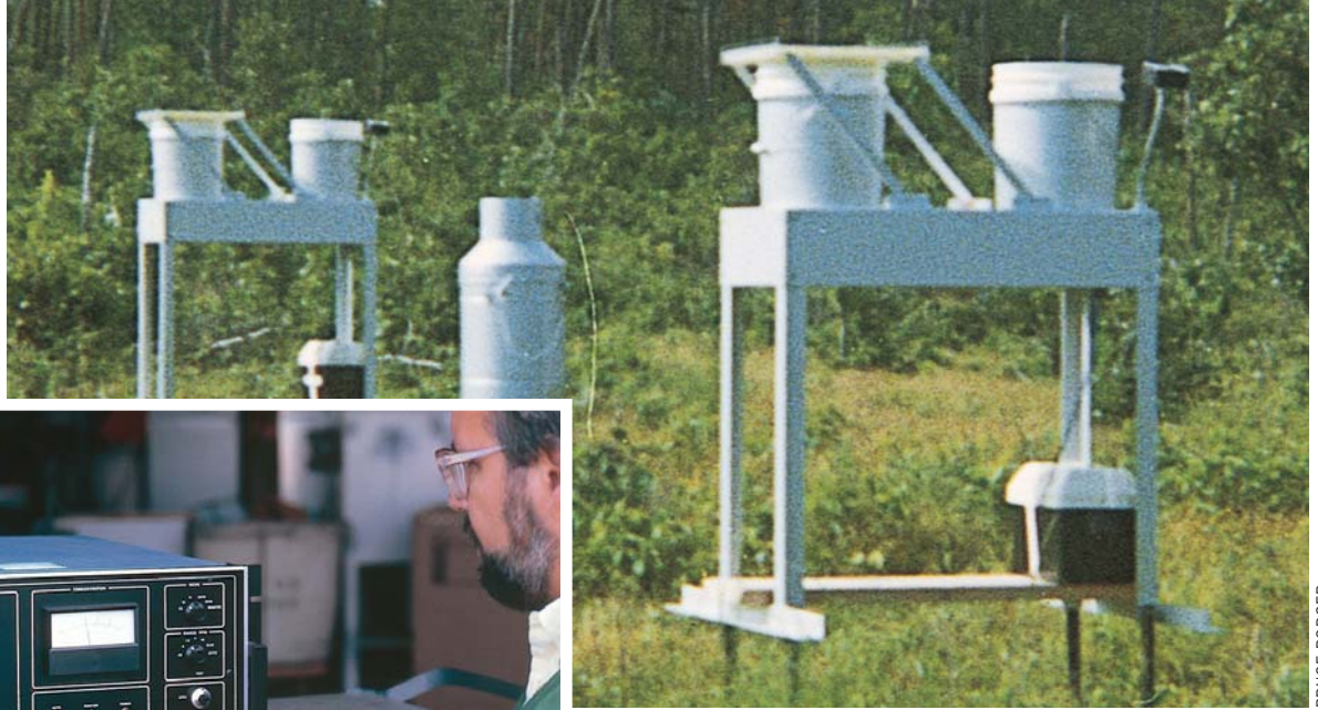
Some of the acid rain test equipment was already available, like the sulfur dioxide analyzer to the left and simple rain gauges. Other tools were invented to match the need. Buckets with automatic lids that shifted as the weather changed caught samples of rainfall, dust and particles for analysis.
