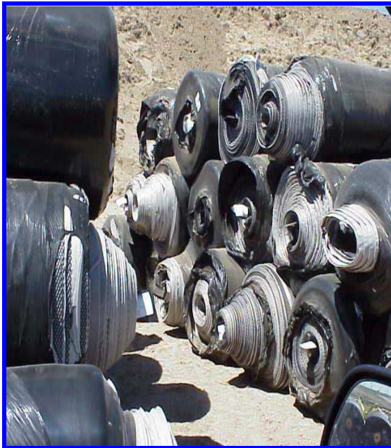
Disposal Site Liner Fabric Source: ThermoRetec
