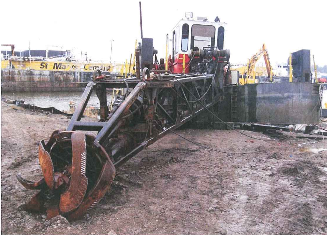
Figure 2. 8-inch hydraulic dredge.
