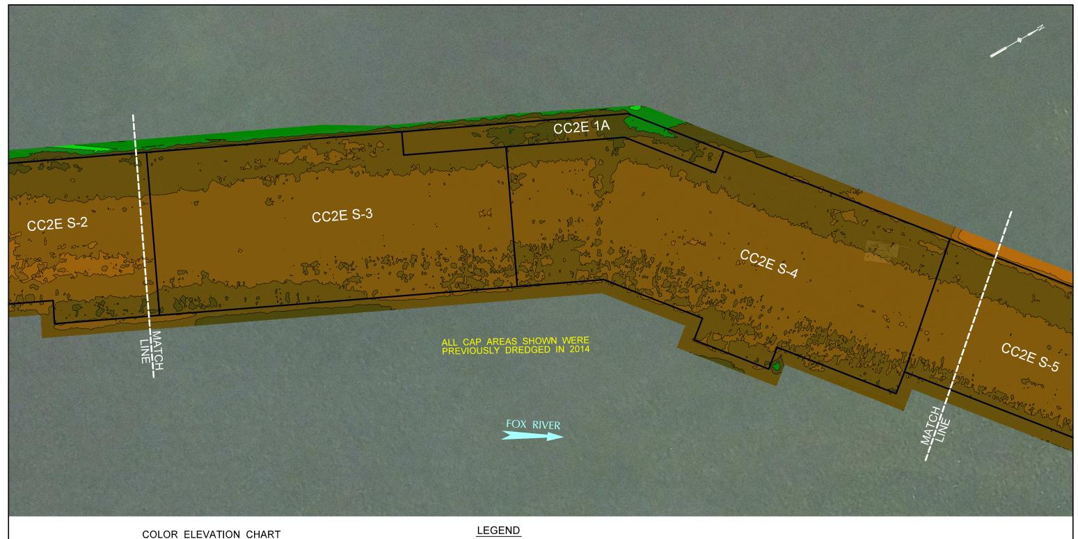
COLOR CONTOURS SHOWN REPRESENT THE OCTOBER, 2017 TOP OF ENGINEERED CAP ELEVATIONS. AVERAGE TIDE ELEVATION DURING TIME OF SURVEY WAS 580.30'.
