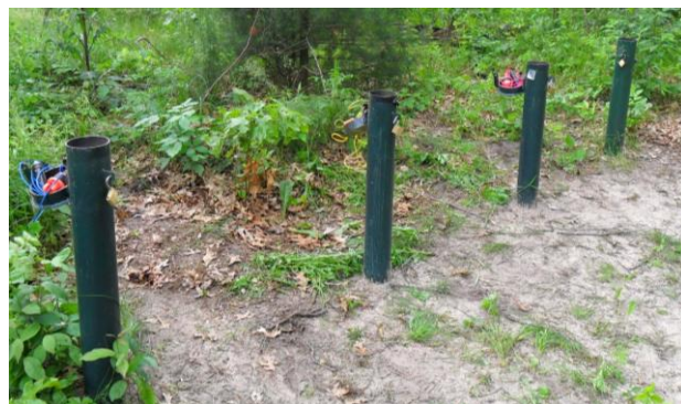
Nestled piezometers installed for monitoring groundwater levels and sampling for groundwater contaminants near Spring Green. Photo: Blake Russo-Nixon.
