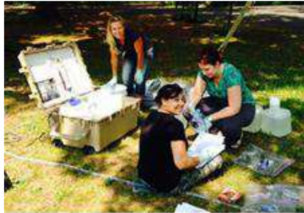
DNR water supply specialists test a new water supply sampling method developed by the State Laboratory of Hygiene. The method will help public water systems distinguish whether the source of bacterial contamination is in the groundwater or from within the water system.
