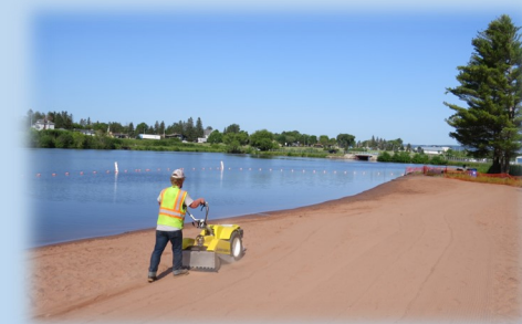
A beach groomer is in use to keep the beach free of debris and potential sources of E. coli bacteria.
