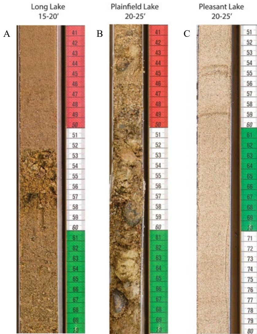
Figure 19. Examples of typical coarse-grained sediment from direct push samples (scale in cm). (a) Long Lake: interbedded sand and gravel in core LL-09 (b) Plainfield Lake: sandy gravel in core PFL-14 (c) Pleasant Lake: well-sorted sand in core PSNT-07.
