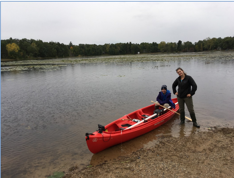
Figure 52. Canoe instrumented with EM-31 conductivity meter, depth finder, water temperature and quality instruments, and Go Pro video cameras.
