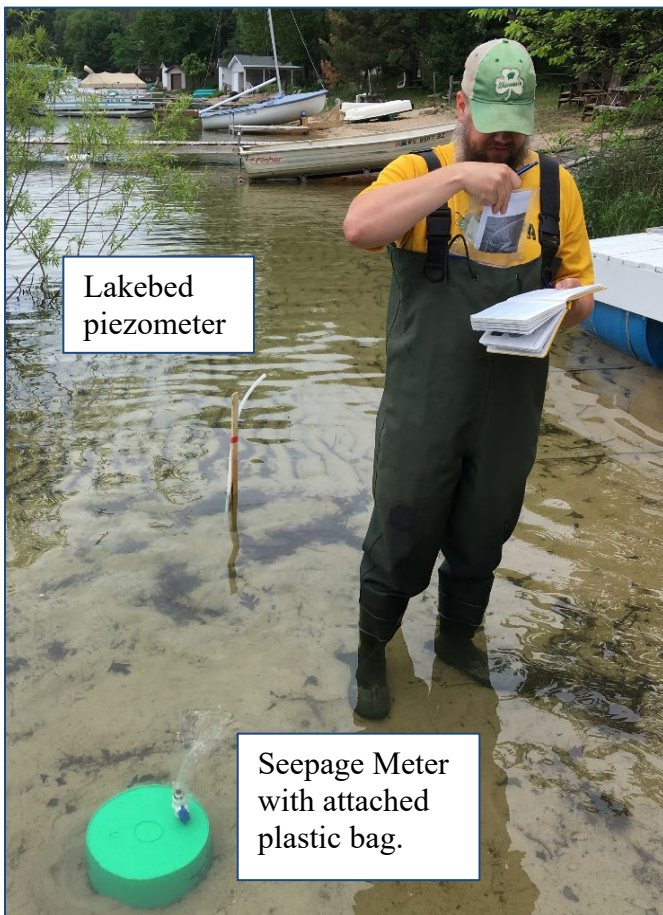
Figure 47. Lakebed piezometer and seepage meter installation
