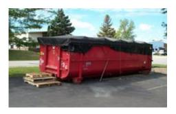
Tarped luger boxes can only be on site during active construction, otherwise must have permanent covers, no rusting, holes, or valves to qualify for No Exposure Certification.
