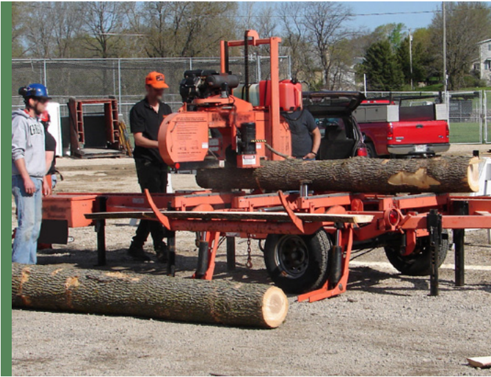
Sawing small ash with a portable sawmill.
